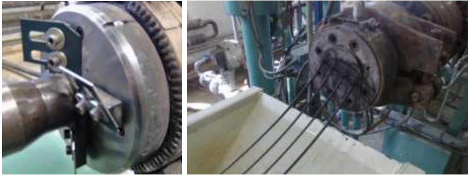
Dry granulation and strand die methods at PEMU
