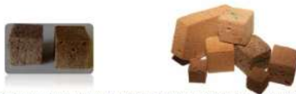
Soft Polyurethanes foams by UNIPi with lignin content 5-13%, total content of renewable material over 40%
